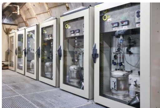
Figure 11 - Cabinets for simultaneous sampling of pore water, dissolved gasses and analyses of geochemical parameters at in-situ conditions, to study pore water geochemistry around the PRACLAY gallery.
