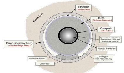
Long-term safety function of the overpack: total containment of the radionuclides during at least the thermal phase by preventing contact between the wasteform and the porewater coming from the host formation.
