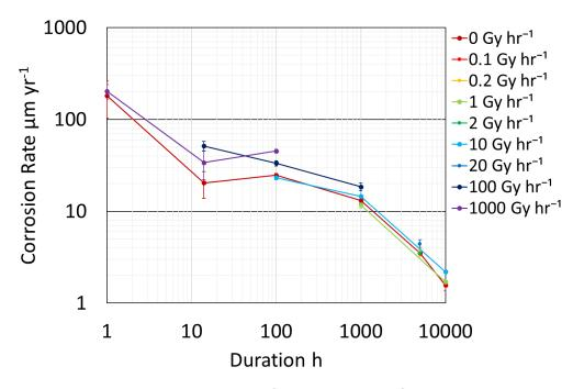
Average corrosion rate of carbon steel for set dose rates
