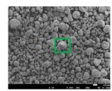
Addition of Cr to the SiC powder (ball milling)
