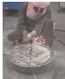
Cutting &amp; dismantling of pellets
