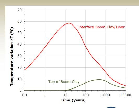
Example of Spent Fuel – UOX50 for a disposal at HADES URL depth where initial temperature is about 16°C
