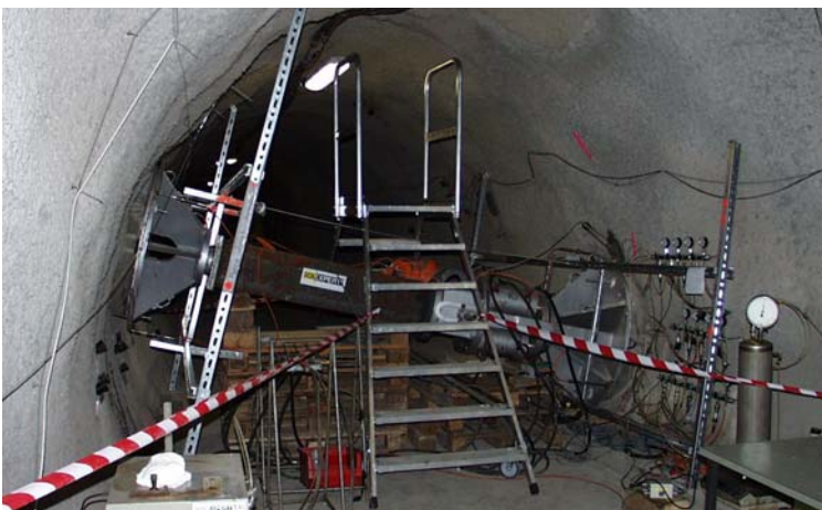
Photo 1: Complete test setup of the load plate experiment [4, 5]
