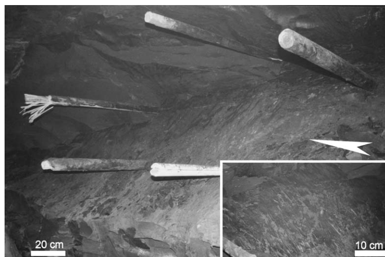
Fig. 7. Pictures of the large shear planes. One can see the safety anchors sticking out of the clay (the anchors are pointing towards the Starting Chamber). The surfaces contain clear striations.
