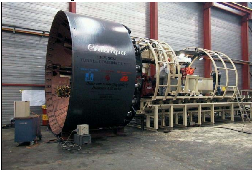
Figure 2. The tunnelling machine used for the construction of the connecting gallery
