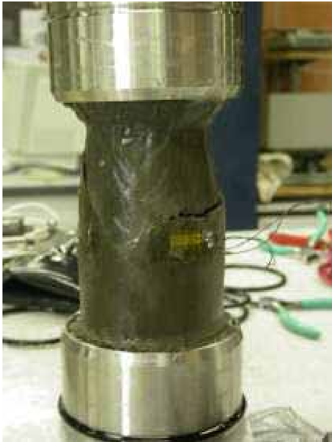
Shear bands observed on sample 1
