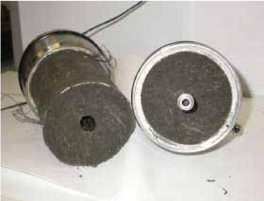
Tensile fracture observed on sample 2 (cored parallel to the bedding planes)
