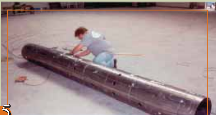
Figure 5: the heater during assembly
