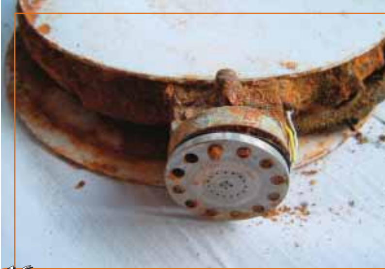
Figures 16: severely corroded Glötzl cells responsible for the release of hydrocarbons in the pore water of the buffer material
