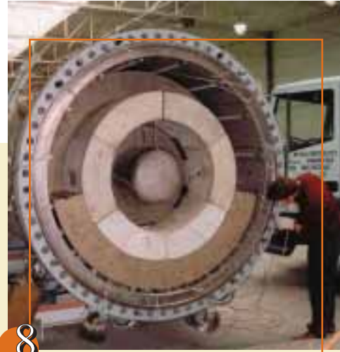
Figure 8: view of the concrete segment and clay-enriched blocks at the extremity of the buffer set-up near the front cover
