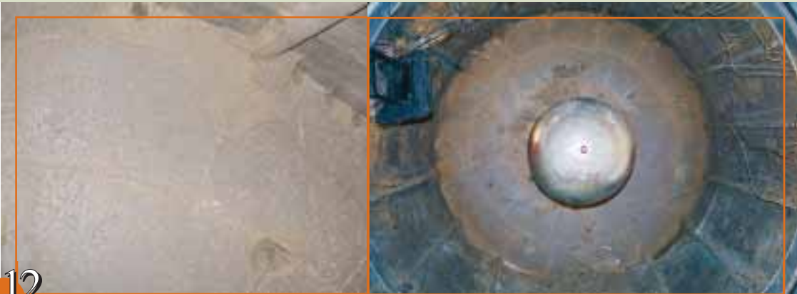
Figures 12: the buffer material filled all technical voids but the joints between blocks were still visible
