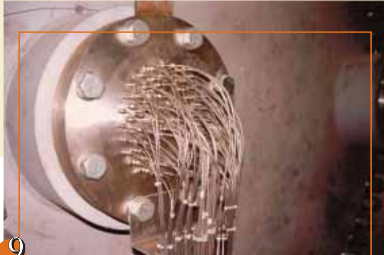
Figure 9: hermetic sealing of the sensor cables
