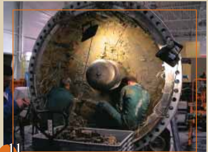
Figures 11: dismantling activities. The movement of sand (white zone) could be observed after removal of the cover (above). Dismantling tasks (below)
