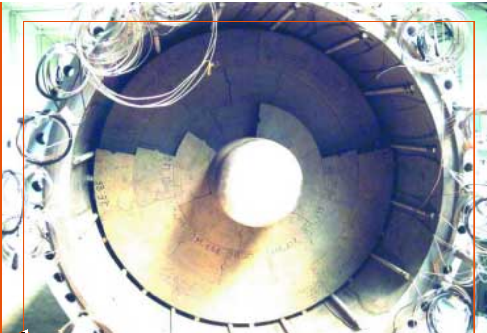
Fig. 1: Mock-up during assembly, with the backfill blocks, hydration tubes and sensor cabling
