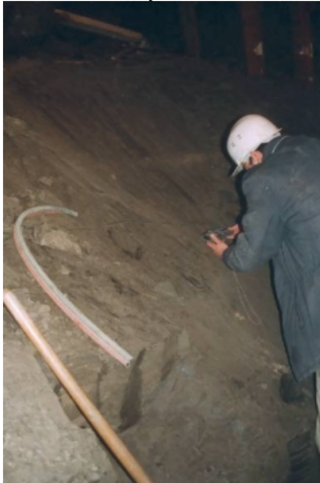
Picture 6: A slickensided surface circular shaped observed in the South starting room (1999)
